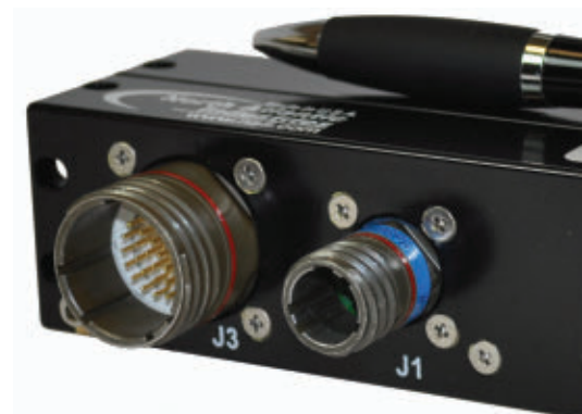
The N1U1A small-form-factor embedded computer from North Atlantic Industries is about the size of a TV remote control, and has applications in unmanned vehicles and vehicle-management systems.
