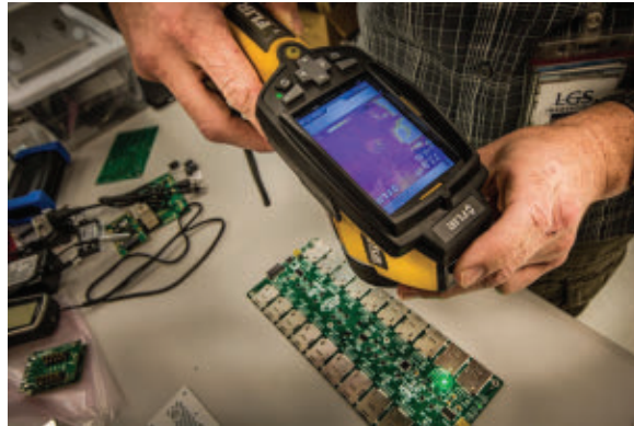
Ryan Straughan, hardware product engineer on the LGS Innovations research and development team, uses a thermal imaging camera to troubleshoot a custom-designed board for situational awareness processing.
